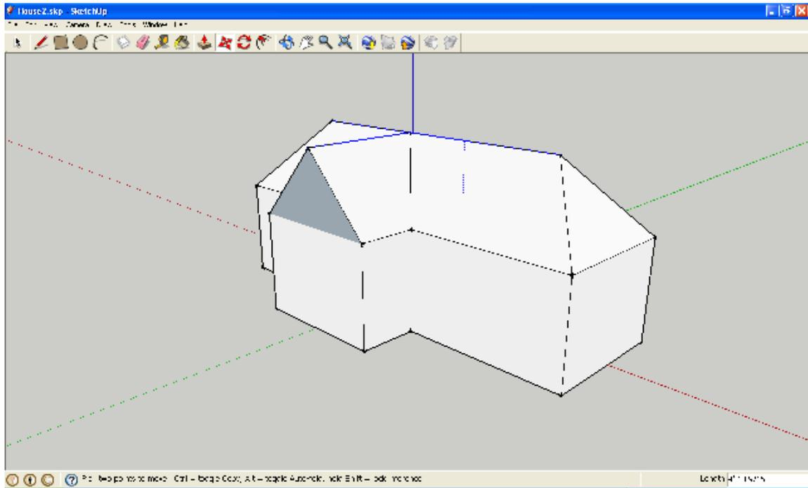
**Fig. 10** Using Push/Pull, with ALT depressed to enable Auto-Folds, creates a roof that is both hipped and gabled.
